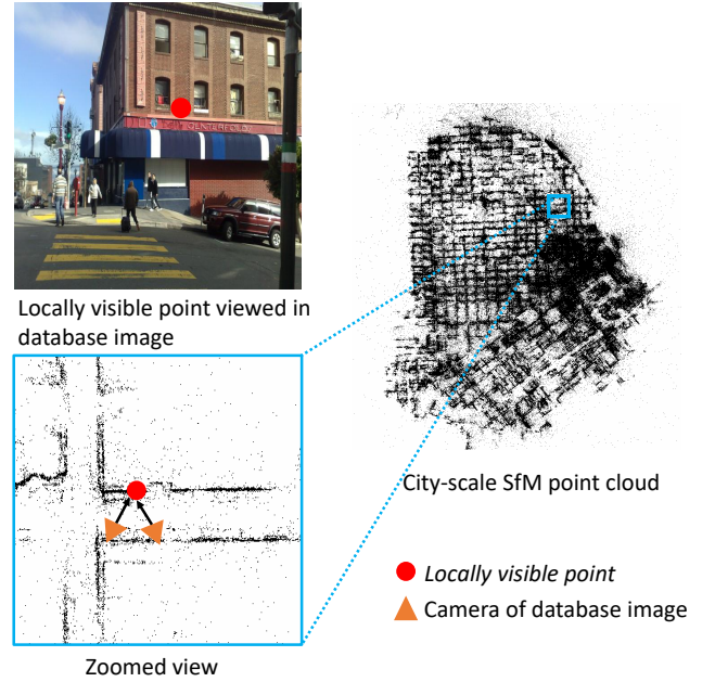
Fig. 3: An illustration of a locally visible point in the San Francisco dataset [4]. A locally visible point (red) is observed by nearby cameras (orange) of the database images.
